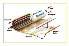
The pre-treated feedwater is pressurised and forced into a series of membrane and pressure vessel assemblies where the separation of pure water and contaminants occurs. Multiple membranes may be used for the higher flow rates and are housed in single or multi-place pressure vessels. RO membranes are available for a wide variety of feedwater types and all have a similar physical structure.
