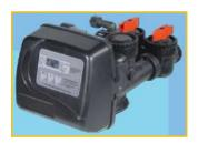
The WS1EI multi-cycle valves are simple, easy to use timer actuated 1" softener or filter flow control valves for 6" to 21" diameter FRP tanks with 2.5"-8 NPSM FRP openings. These versatile valves are primarily designed for commercial applications requiring flow rates up to 102lpm at 103kPa pressure drop. The valve uses a 1.05" riser tube and comes with an upper bayonet type screen. Standard supply includes a bypass assembly as standard to simplify service requirements.
