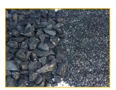
Anthracite Filter Media is sourced from anthracite which yields the highest percentage of carbon. It is then hydraulically classified to reduce mineral matter and ash to a minimum, and finally screened and washed to ensure suitability for filtration purposes.
