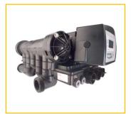
The Magnum Cv is a 1.5" flow control valve is moulded from Noryl available with an external flow metering turbine. Used for commercial and industrial applications, the valve provides for flow rates up to 285lpm @ 103kPa pressure drop. All options are ordered separately. Filter application order backwash flow control separately.
