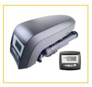
The 263 Performa model is an automatic 3-cycle 1" Filter valve designed for larger residential and light commercial applications with higher service flow rates to 95 LPM at 103kpa drop and backwash flow rate of 76 LPM at 170kpa drop. The Performa valves are supplied complete with a 400 or 900 Series Control with transformer and have four external ports that allow the valves to be configured to suit most applications.
