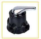
Economical back-washable filter. Simply turn the rotary valve handle to backwash the filter. Complete with backwash flow control and ball valve. Ideal for sites where electric power is not available or for filtering water where minimum backwash waste is required e.g. tank water.
