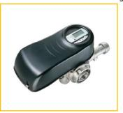
The 150/153-316 Stainless Steel valve is a 1.5", 3-cycle filter valve designed for commercial and industrial applications with flow rates to 216lpm @ 103kPa pressure drop. The valve is 316 grade stainless steel, piston operated and is available in top or side mount formats
