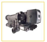
The Magnum Cv is a 1.5" flow control valve is moulded from Noryl available with an external flow metering turbine. Used for commercial and industrial applications, the valve provides for flow rates up to 285lpm @ 103kPa pressure drop. All options are ordered separately. Filter application order backwash flow control separately.
