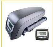
The 263 Performa model is an automatic 3-cycle 1" Filter valve designed for larger residential and light commercial applications with higher service flow rates to 95 LPM at 103kpa drop and backwash flow rate of 76 LPM at 170kpa drop. The Performa valves are supplied complete with a 400 or 900 Series Control with transformer and have four external ports that allow the valves to be configured to suit most applications.
