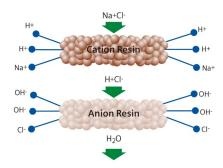
Exchange deionisation systems provide a simple means of producing low conductivity water either directly from a mains feedwater supply or as polishers for reverse osmosis systems. A typical exchange mixed bed deionisation system includes pre-filtration, dechlorination and two resin beds. Options are available for UV sanitation and sub-micron final filtration stages. System capacity will vary according to feedwater conductivity and the amount of ion-exchange resin in the
