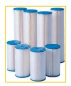
**Pleated sediment filters** are used with high sediment feedwaters and where limited element washing is advantageous. The filter is made in a pleated sheet with an inner core and ultrasonically welded end caps. High pleat count and a rigid inner core reflect the quality and long in-service life of this filter type.
