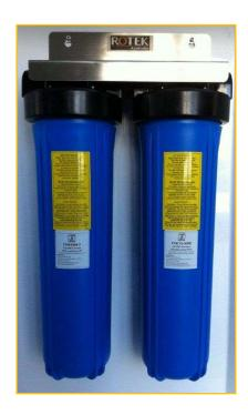
DUO2P-4520 high-flow dual-stage cartridge filtration systems use industry standard 4.5" x 20" injection moulded filter housings mounted on a stainless-steel wall bracket. Systems are supplied configured with filter cartridges to suit specific applications.
