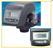
The 255 model is an automatic 5-cycle 3/4" softener valve designed for residential applications with service flow rates to 58 LPM at 103kpa drop. The 255 Valve uses a standard 1.05" riser tube. The 255 Valves are supplied complete with a 700 Series Control with transformer, Air-Check Assembly, Severe-Service Valve Disks and Tank O-ring as standard. The appropriate brine injector and backwash flow control restrictor are supplied to suit each assembled system.
