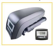
The 268 Performa model is an automatic 5-cycle 1" softener valve designed for larger residential and light commercial applications with higher service flow rates to 95 LPM at 103kpa drop and backwash flow rate of 76 LPM at 170kpa drop. The Performa valves are supplied complete with a 700 Series Control with transformer and has four external ports that allow the valves to be configured to suit most applications.
