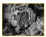
**GC1200 and 1200N series** are microporous, acid washed (N type), pH stabilised coconut-based media used to remove low molecular weight organic micro-pollutants, ozone, and chlorine-based sanitisers from feedwater sources.
